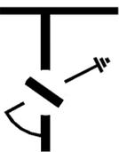
Open the load break switch and the earthing switch before carrying out the work described in the manual.
